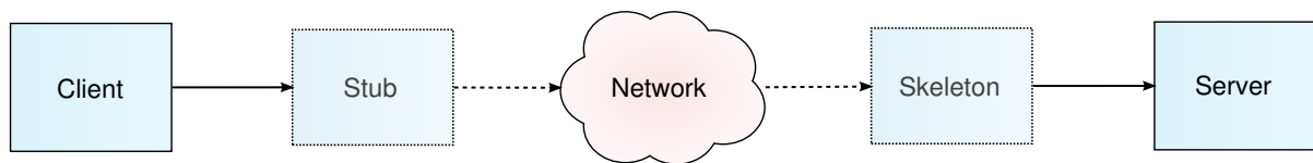
Figure 2.5: Structure of Remote Message Invocation: Method calls from Client to Server are routed over the network through automatically generated proxies called Stub and Skeleton.
